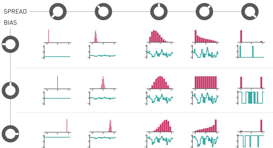
**M. Horizontal and vertical “steppiness”** of the generated voltages. At 12 o'clock, generates the typical S&H steps. Turn CCW to generate smoother edges, then random linear segments, then smooth random curves. Turn CW to quantize the generated voltages to a scale, then to progressively strip the scale of its notes until only the root note remains.
