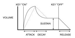
The ADSR envelope can be most easily visualised by considering the amplitude (volume) of a note over time. The envelope describing the "lifetime" of a note can be split into four distinct phases:
