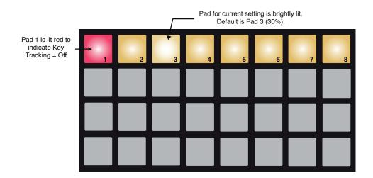
Only the top row of the grid is active in this View. Press one of Pads 1 to 8 to select the degree of Filter Key tracking required, according to the table:
