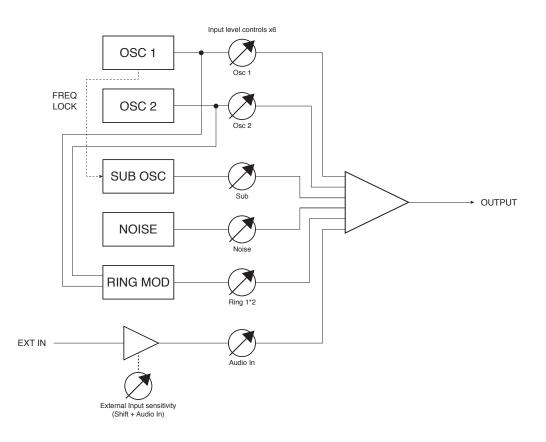
The outputs of the various sound sources can be mixed together in various proportions to produce the overall synth sound, using what is essentially a simple 6-into-1 mono mixer.
