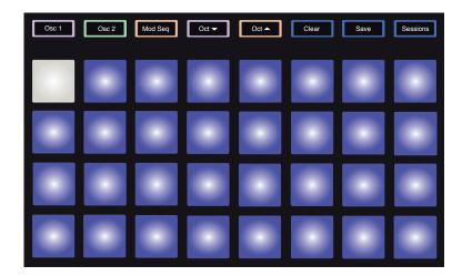
The two pages are selected with the Oct  $\checkmark$  and Oct  $\land$  buttons 12. In Page 1, Oct  $\checkmark$  is illuminated bright white and Oct  $\land$  dim white. Pressing Oct  $\land$  will open *Patch View Page 2*.
