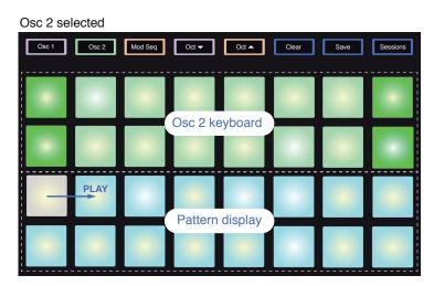
The Osc 2 level control in the Mixer section 24 must be turned up and Paraphonic mode 2 selected (by pressing **Shift + Scales**) in order for Oscillator 2's notes to be audible. Note that the **Scales** button is illuminated bright white when Mode 2 is active.
