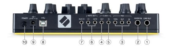
1 **LINE OUT** – the main (mono) audio output on a ¼" TRS jack socket. Max. output level is +10.5 dBu. The output is pseudo-balanced (ground compensated) and may be connected to equipment with either balanced or unbalanced inputs.
