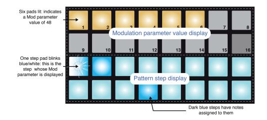
Pressing Mod Seq 5 opens Modulation Sequencer View:
