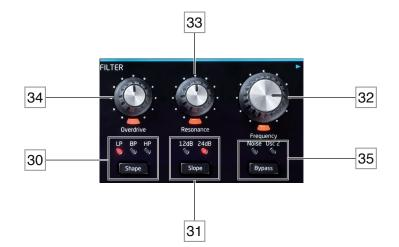
The sum created in the mixer from the various signal sources is fed to the Filter Section. Circuit Mono Station's filter section is both simple and traditional, and can be configured with only a small number of single-function controls.
