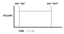
A piano note quickly attains full volume after a key is pressed, but gradually falls in volume to zero after several seconds, even if the key is held.
