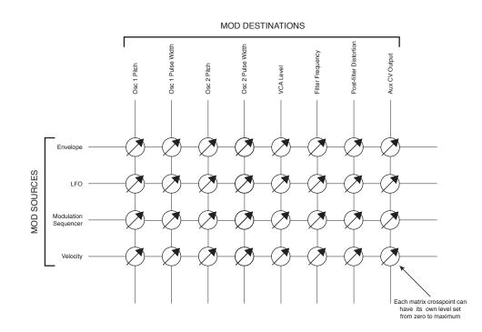
The Modulation Matrix may be visualised as a system for connecting controlling sources to a specific area of the synth. The matrix has four sources and eight destinations and thus has 32 crosspoints. The matrix is *variable*.
