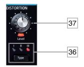
The **Type** button <u>36</u> selects one of three analogue distortion types, simply referred to as I, II and III:
