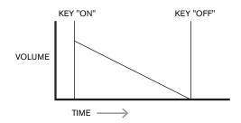
A string section emulation only attains full volume gradually when a key is pressed. It remains at full volume while the key is held down, but once the key is released, the volume falls to zero fairly slowly.
