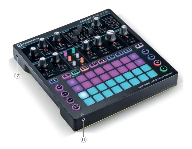
(1) (Headphones) – connect a pair of stereo headphones to this 3.5 mm TRS jack socket. The headphone amplifier can drive +10.5 dBu into 150 ohms.
