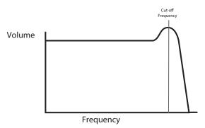
In addition to the traditional low-pass filter type, there are also high-pass and band-pass types. On Circuit Mono Station, the Filter type is selected with the **Shape** switch 30.
