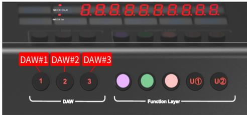
In order to allocate the right DAW to the right DAW button (above), we're going to need to use the iMAP. It is always best to always have the iMAP running in tandem with the V1-M. In this way on-the-fly changes can be made with immediate effect.
