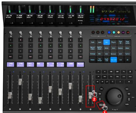
You can also assign CC, Note, pitchbend values and MIDI channels to the master fader in Assign mode via the iMAP.
