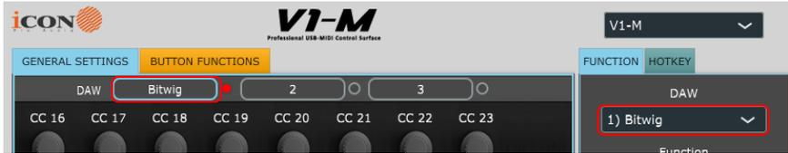
So, you've downloaded, installed and opened the iMAP. You will see the three DAW buttons on top of the iMAP. These correspond to the three DAW buttons on the V1-M.
