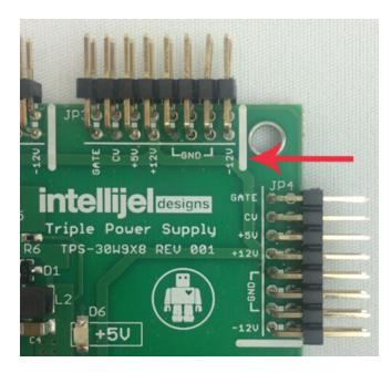
The other end of the cable, with a 16-pin connector, connects to the power bus board of your Eurorack case. Ensure the red stripe on the cable lines up with the -12V pins on the bus board. On Intellijel power supplies the pins are labelled with the words "-12V" and a thick white stripe.
