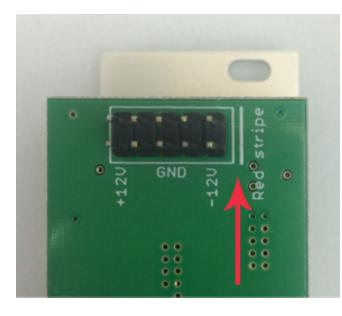
Ensure the 10-pin connector on the power cable is connected correctly to the module before proceeding. The red stripe on the cable must line up with the -12V pins on the module's power connector. The pins are indicated with the label -12V, a white stripe next to the connector, the words "red stripe", or some combination of those indicators.
