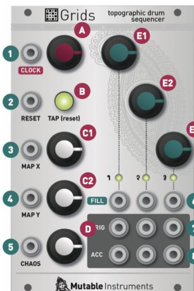
**A: Internal clock rate.** Ranges from 40 BPM to 240 BPM. When turned fully counter-clockwise, the internal clock is disabled and the unit expects a clock signal on its CLOCK input.
