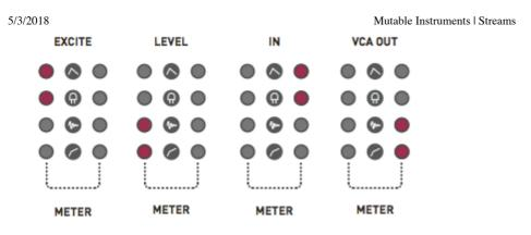
Note that the arrangement of the LEDs mirrors the arrangement of the physical inputs/outputs of the channel 1 of the module.
